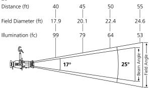
For illumination with any lamp, multiply the candlepower of a beam spread by the multiplying factor (mf) shown for that lamp.
