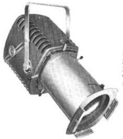
Patt.253 Profile 2000 Watt 24 degree beam angle with 4 built-in beam-shaping shutters, built-in 18 leaf iris diaphragm and internal terminal block.
