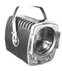
Patt.243BP Fresnel Spot 2000W CP/41 Halogen lamp. G38 base Lead-screw focus. 250mm diameter lens. 16 degree / 50 degree variable spread 430mm length. 14kg
