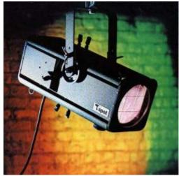
T spot is based upon a computer designed optical system which achieves 40% increase in light over other 1000 watt halogen profile spots.; also T-spot incorporates a beam shaping shutter assembly affording an infinite permutation of shape and the projection of hard edges, soft edges, or a mixture of both hard and soft edges simultanuously. This allows precise cut off on one or more sides, with others merging into adjacent beams and patterns of light.
