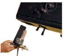
A removeable lamptray holds the 1000 watt tungsten halogen lamp. Spare lamptrays are available to overcome the problem of replacing a failed hot lamp, quickly without altering the orientation or adjustment of the spotlight.
