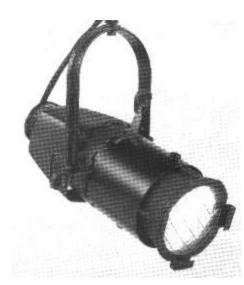
A wider angled ellipsoidal reflector spotlight with 45° cut-off, using dual 6" diameter lenses and focal length 9".
