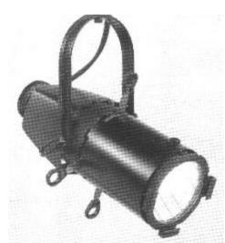
A narrow beam ellipsoidal reflector spotlight with a 21  $^{\circ}$  cut-off, with dual 6" diameter lenses and focal length 16".
