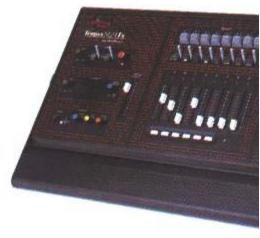
This compact, lightweight control offers a choice of 24, 48, 72, 96 or 120 channels, and the facility to record up to 199 lighting states. It can be used as an independent new system, or as an extension to an existing manual system.
