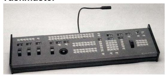
Taskmaster memory control system for Showchangers, complete with disc drive, 2 metres of mains cable and 8 metres of data cable.
