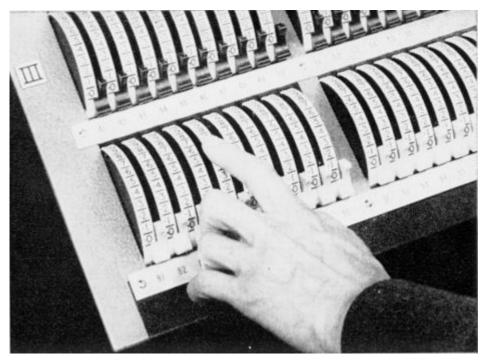
On System LP the dimmer scale carries two internal indicator lam white. In addition, the scale can spring to use it as a push button (photo left). The levers mount at and 4½" vertically. All confusion another is avoided by the special dimmer knob which not only profinger to rest but places it over the
