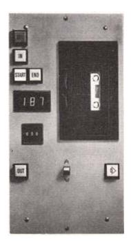
This allows the content of the entire Core Store module to be transferred to and from a magnetic tape cassette for repertoire storage.
