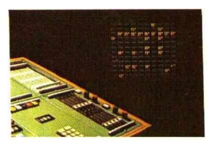
Active or preview mimic display can be either above-zero indication, or a colour and/or monochrome video display showing precise intensity
