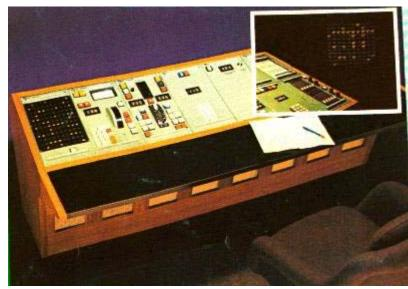
The Modular Memory System consists of a number of modules, each providing complementary or alternative operational facilities, which all plug into a common digital data link. For 80 up to 360 control channels, with only two module types repeating for each multiple of 120, or less, channels.
