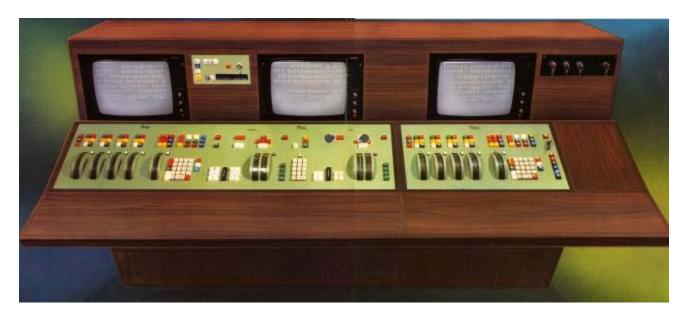
**LIGHTBOARD** allows the simplest or most complex lighting pictures to be moved at one or many varying interweaving speeds.
