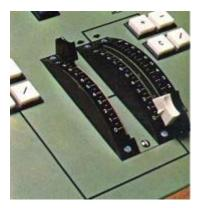
Another valuable performance facility is Sequence, which automatically recalls the next cue from the memory on completion of a dipless or contoured crossfade. Nor are essential ancillary controls forgotten - there are ten foldaway fader levers for both pile-on and inhibitor mastering of ten groups selected on a pin-patch matrix.
