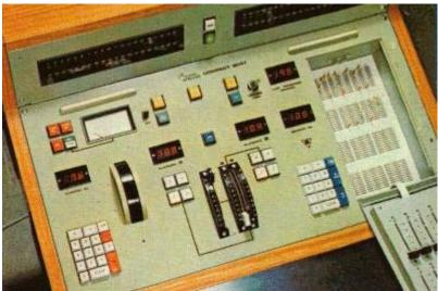
Compact has many advantages over the multi-preset, multi-group lighting controls which it succeeds. It is much smaller and fully mobile. It is also far faster in rehearsal and far more accurate in repetition for each performance. Moreover, the memory, equivalent to 130, 200 or 260 presets, enables the operator to concentrate on the visual effect of each lighting change, instead of having to reset fader levers to intensity levels hastily scribbled at rehearsals.
