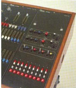
This optional module features two sophisticated effects generators, plus a four frequency band sound to light convertor. The two effects generators each have 7 different modes for variable speed chase and cycle functions, including progression triggered by the bass beat of an external audio signal. The vertical columns of push switches and a flash push select the nine group masters of the AMC master module to any of the effects sources.
