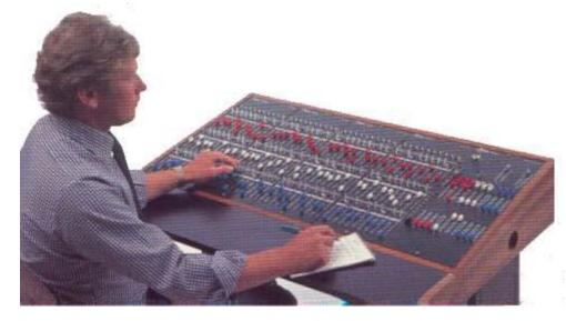
Multi-preset, multi-group desks are based upon 10channel 3-preset modules, a choice of Master modules both with a dipless crossfader for 9 submaster groups, and an optional Effects module. These various modules, also including selectable inhibit master/independent arouping, combine to form the most comprehensive manual control system for as few as 20 up to a maximum of 120 control channels.
