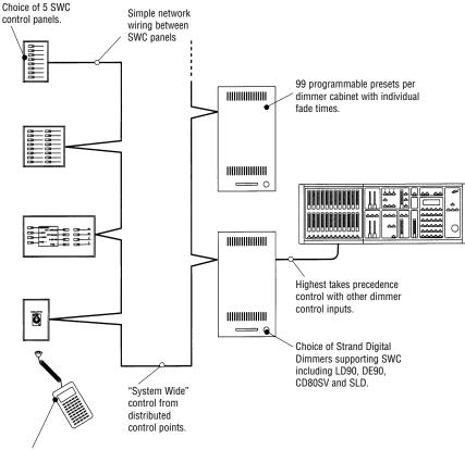
Hand held control for rigging, focusing and programming.
