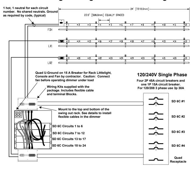
Note: Electrical panel, wiring, conduit and circuit breakers supplied and installed by contractor. Not included with system package
