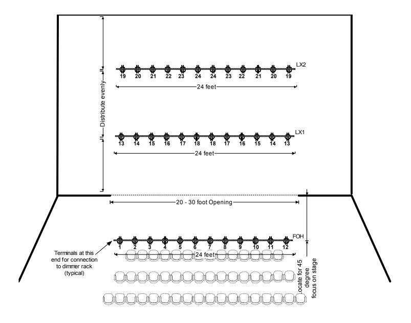
Note: This is only a guide for circuit placement distribution with this package system. If other project drawings specify this information it should be confirmed which is accurate.
