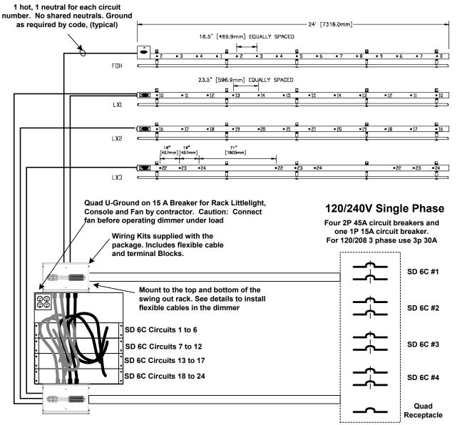
Note: Electrical panel, wiring, conduit and circuit breakers supplied and installed by contractor. Not included with system package
