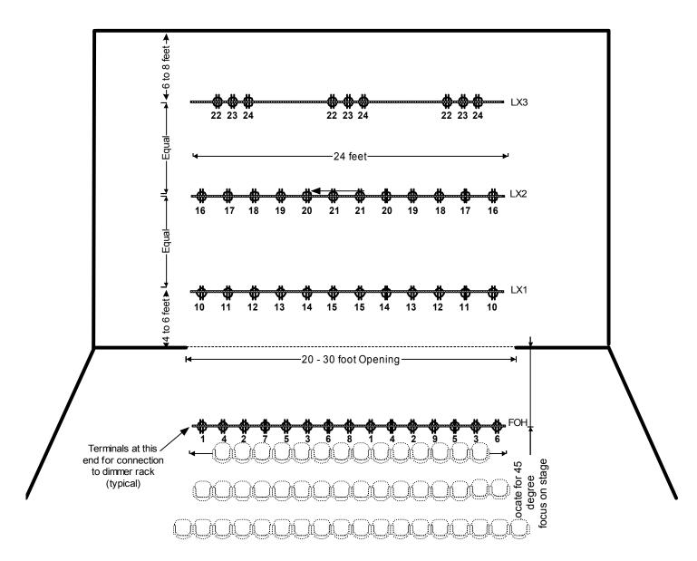
Note: This is only a guide for circuit placement distribution with this package system. If other project drawings specify this information it should be confirmed which is accurate.
