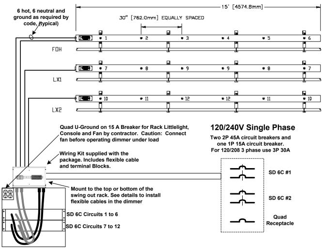
Note: Electrical panel, wiring, conduit and circuit breakers supplied and installed by contractor. Not included with system package
