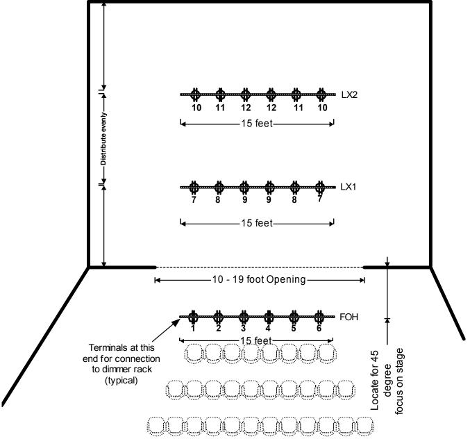
Note: This is only a guide for circuit placement distribution with this package system. If other project drawings specify this information it should be confirmed which is accurate.
