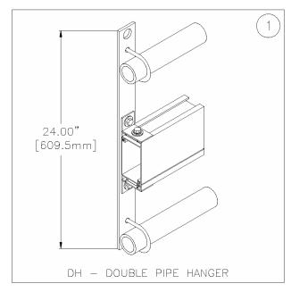
Single Pipe Hanger, (Load method #1), (can be used as Grid hanger above pipe) and Double Pipe Hanger are designed to carry fixture load on the pipe only.
