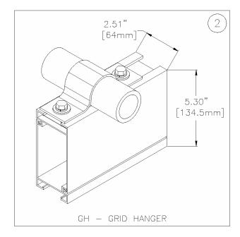
Flat Hanger and Grid Hanger are not designed to carry fixture loads.
