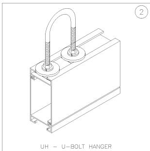
Rod Hanger and U-Bolt Hanger, (Load method #2) are not designed to carry fixture loads.
