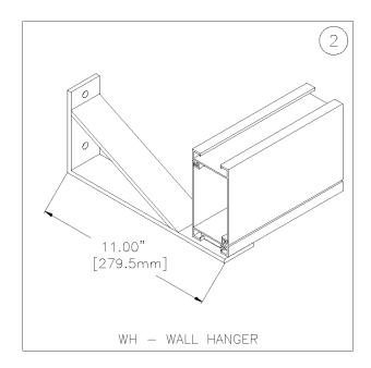
Vertical Pipe Hanger and Wall Hanger are not designed to carry fixture loads.
