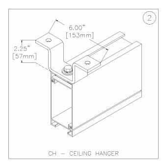
Bolt On Hanger and Ceiling Hanger are not designed to carry fixture loads.
