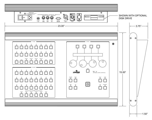
The MLC 16 control console is designed to communicate with all DMX512 intelligent luminares. The MLC 16 is delivered preprogrammed for several of today's most popular intelligent products and may be easily configured, by the user, for other fixtures. Equipped to address multiple personalities, the MLC 16 gives the user the ability to control a variety of devices from different manufacturers, all at once.
